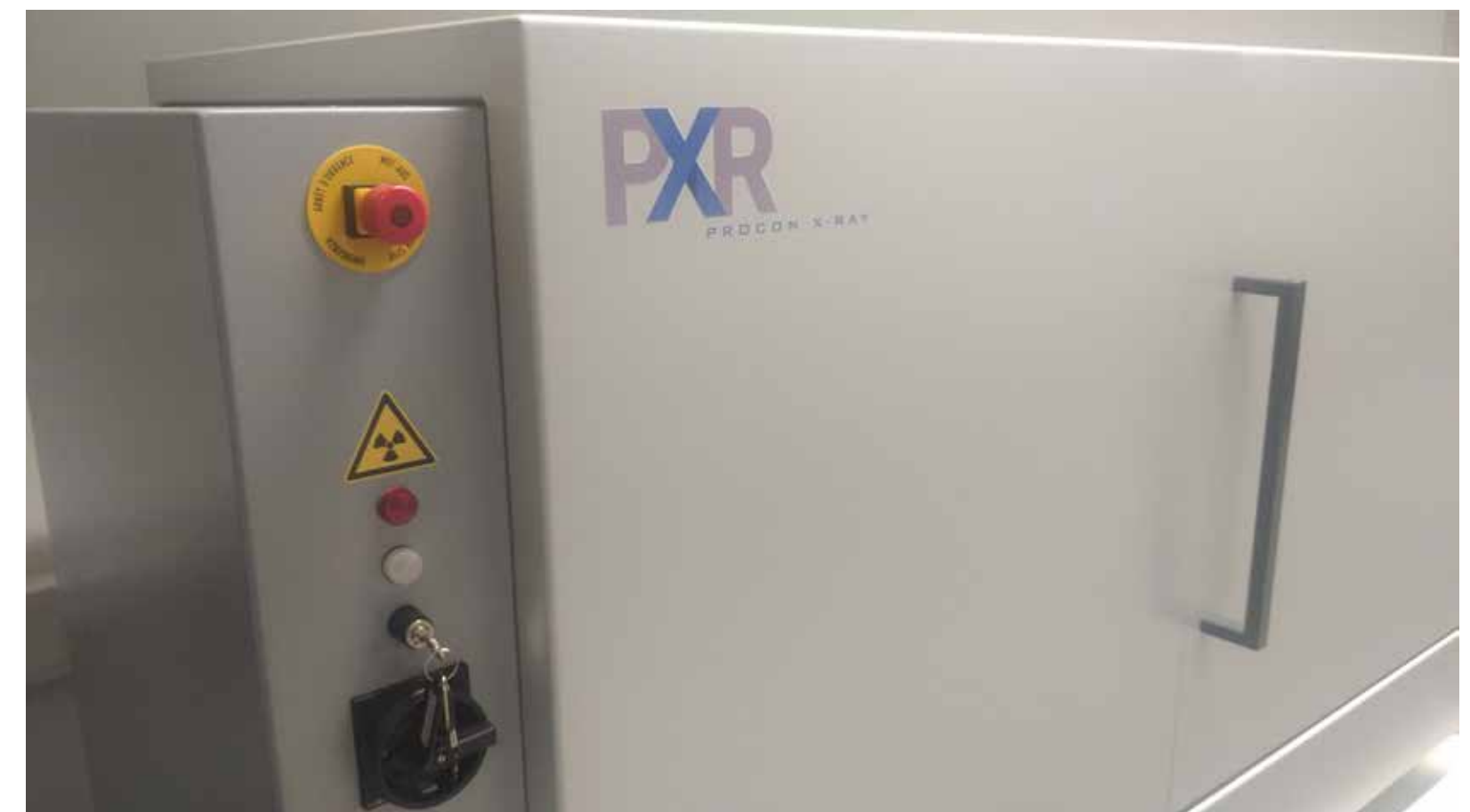
PXR CT-Compact 130 Röntgenschränk (ProCon x-ray GmbH)
