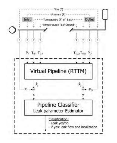
Model-based leak detection and leak location using the Extended RTTM (E-RTTM) method.
