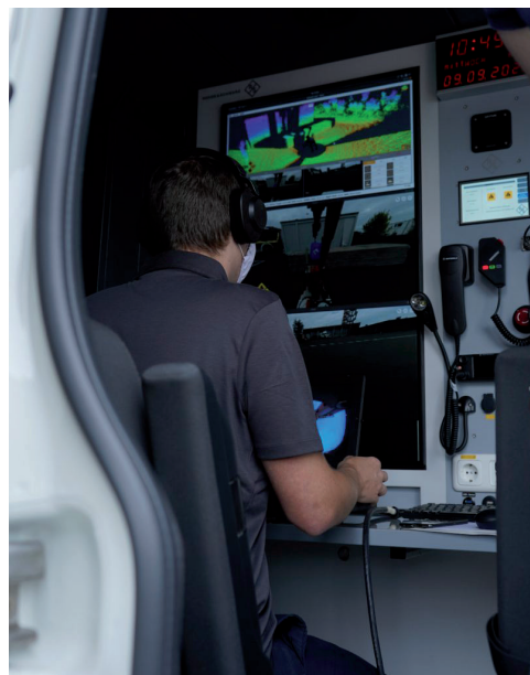
Fig. 2: One of the two workplaces for the robot operator in the Rob-LW (mobile transporter of the fire brigade).
