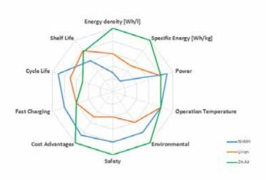
Fig. 1: Comparison of various battery technologies
