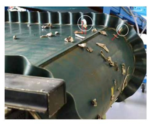
Fig. 1: Separating rare earth magnets with eddy current separators
