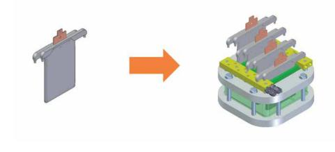
Fig. 1: Schematic drawing of the modularly constructed electrolyser with four individual cells.
