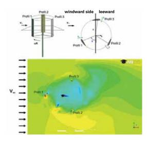
Fig. 1: H-rotor with 3 profiles
