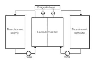
Fig. 1: Schematic Sketch of a Redox-Flow Battery
