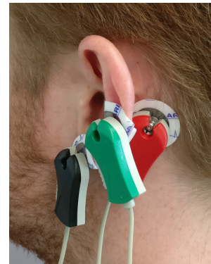
Figure 10: Setup for measuring the activity of the posterior auricular muscle. The electrodes are positioned at the posterior auricular muscle (red), the ipsilateral pinna (reference, green) and ear clips for grounding (black).
